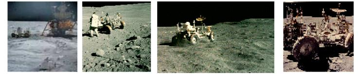
The Lunar Rover has steel-wire tires to get a good grip in the moon dust and an electrical motor in each hub, top speed 14 km/h. The driver has one hand on the lever which serves as a steering wheel, gear shifter and accelerator. A computer replaces the compass, the Moon has no magnetic field.
