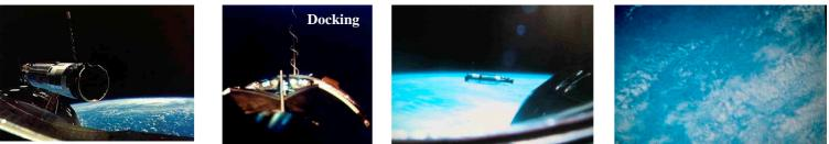
Gemini 8 and Agena meet. The Gemini 8 crew have problems: while the vehicles are connected one of Gemini 8's thrusters for rolling causes a rotation which quickly increases. The strain threatens to break the front part of Gemini 8. Armstrong undocks and finally manages to stop the spin.
